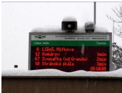
Electronic information panels, on-line vehicle positions
